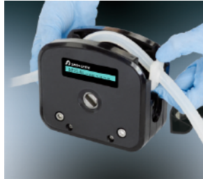
B. Put the tubing with cartridge or connector into pump housing.
