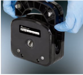
A. Lift both side levers, take off the upper block.
